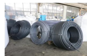
Underground internet tube (SCCP, Bulgaria)
